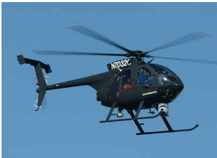
Boeing's Unmanned Little Bird has performed shipboard autonomous takeoffs and landings off the coast of Florida. Photo courtesy the Boeing Co.
