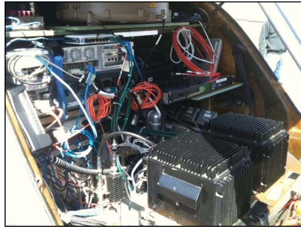
Figure 1: Interior of Proxy's payload bay showing a payload of 5 sensors and processors, 5 communications systems, and Proxy's Virtual Pilot.
